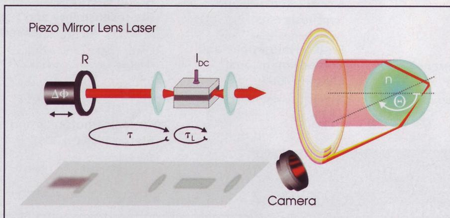
**Figure 1.** This incoherent semiconductor laser source uses the well-controlled feedback properties of an external cavity configuration with a piezo translator-mounted mirror (R) for rainbow refractometry on a liquid droplet.
