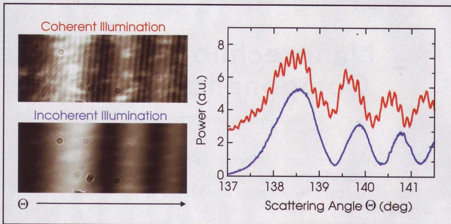
Figure 2. The camera pictures on the left contrast the smooth intensity distribution for coherent illumination (coherence length 8 m) with that for incoherent illumination (coherence length 120  $\mu\text{m}$ ), and the graphs confirm these differences.
